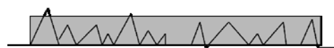
Complete wetting out of surface with adhesive results in superior mechanical and chemical forces and overall adhesion.
