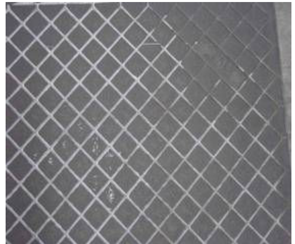
Kiln release easily visible on back of tile
